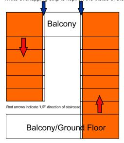
11. Measure and cut Stickymat to fill balcony void area. Measurement must include the total width of the overlapping strip so that the adhesive side covers the lap completely
