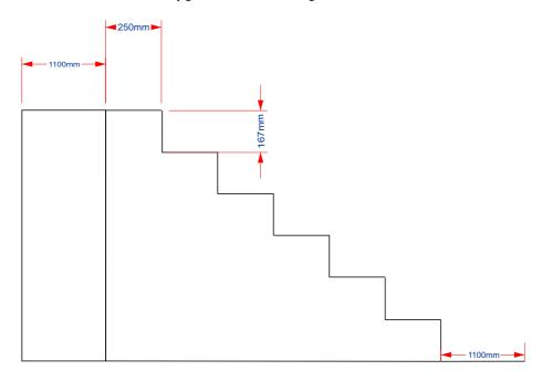
3. Add measurements of treads, risers and balcony/ground floor widths then cut mat to size
