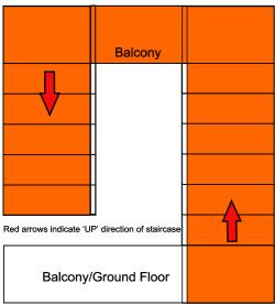
13. Where you come to the end of a roll that does not cover a full flight of stairs, always finish at the bottom of the riser
